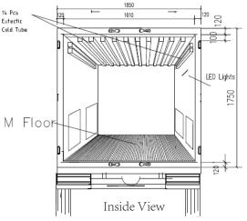
Box Overall Dimensions: 2400 (L) X 1850 (W) X 1750 (H) mm Box Volume: 5.2 m<sup>3</sup> Refrigeration: 14pcs eutectic coldtube beams Transport Temp. Required: -40 °C Compressor: Bitzer 3P Power Supply: 380V (50Hz/60Hz) / 3 Phase Charging Time: approx. 6 ~ 8 Hours Refrigerant: R404a
